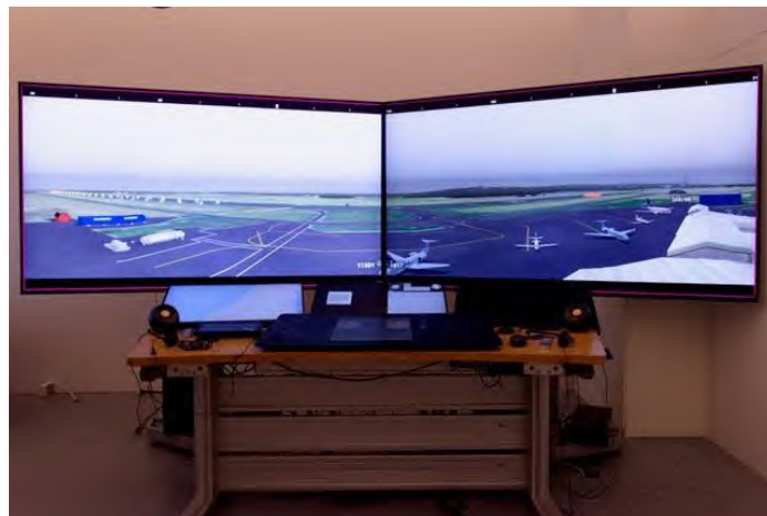
Figure: MRTM2 – comprising of 2 (82”) screens, positioned in landscape mode
