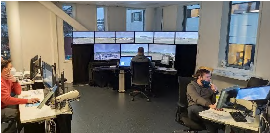
Figure: Validation setup with two MRTMs, two ATCOs and one supervisor
