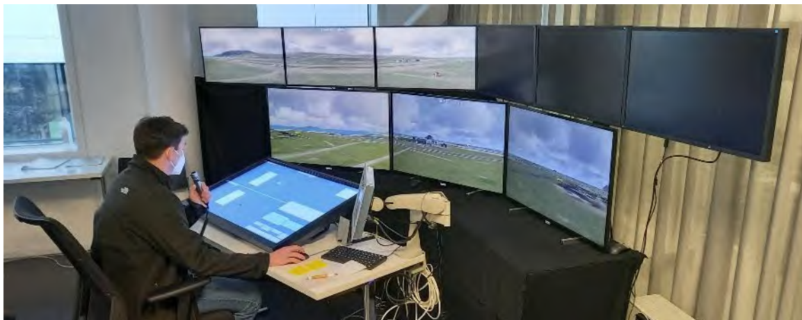
Figure: ATCO in MRTM2 with the hand-held microphone. The mic had two buttons under each other, with the same surface and shape, so haptic differentiation was difficult.
