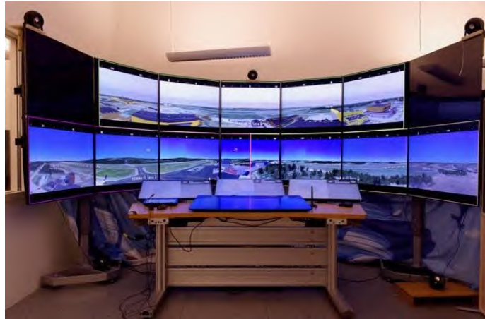
Figure: MRTM 1 – comprising of 7 (55”) screens, positioned in portrait mode
